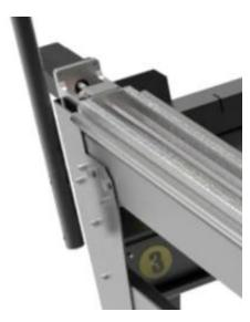
Step10: Position the support frame to the machine side and secure.
